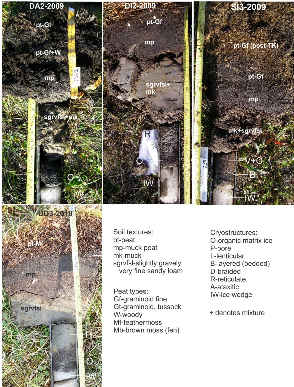
Fig. SI12. Examples of soil profile by degradation stage. Coding for soil textures, peat types, and primary cryostructures given in legend.
