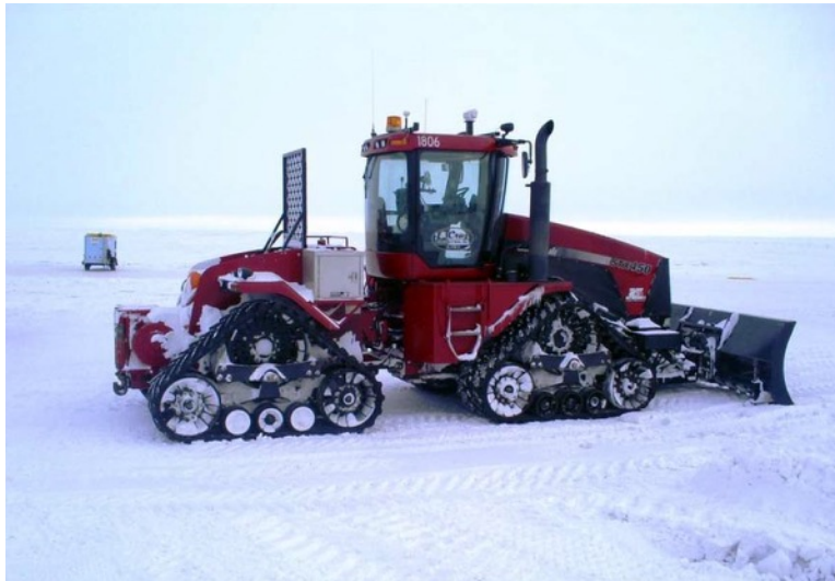
Figure A3: Steiger tractor used to haul camp trailers and other vehicles and equipment . The plan of operations anticipates nine Case/Steiger tractors per crew. (Photo: Alaska Department of Natural Resources)
