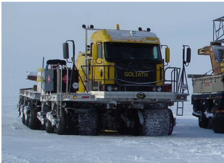
Figure A4: Rolligons are vehicles with large low-pressure tires used by the oil industry in Canada and Alaska. The plan of operations lists one Rolligon per crew. (Photo: Alaska Department of Natural Resources)
