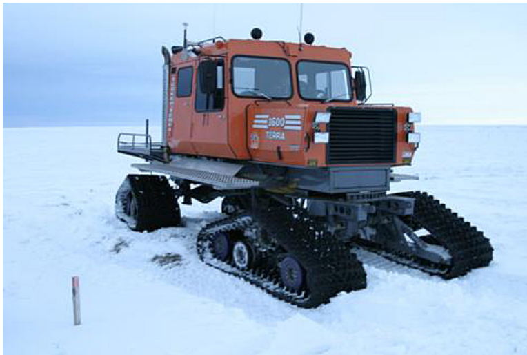
Figure A2: Tucker Sno-Cat, a cleat-tracked vehicle used to transport workers, prepack snow, and other uses not requiring a heavy vehicle. The plan of operations includes 12 Tucker Sno-Cats, eight Tucker Ice Cats, three Tucker personnel carriers, and a variety of Tucker trailers per crew. (Photo: Alaska Department of Natural Resources)
