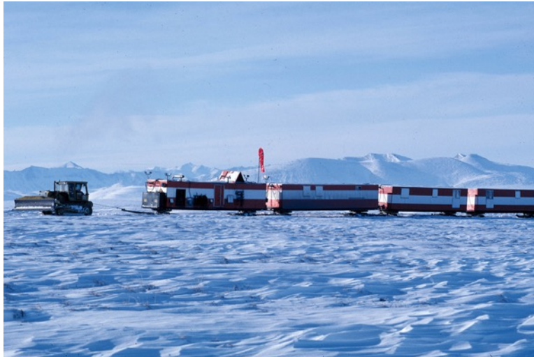
Figure A7: Cat train with sled-mounted camps pulled by a D7 dozer during the 1984–1985 surveys. The plan of operations proposes one 150-person sleigh camp per crew. The vehicles required for the mobile camps consist of 8–10 strings of 5–8 sleds pulled by large tractors. (Photo: U.S. Fish & Wildlife Service)
