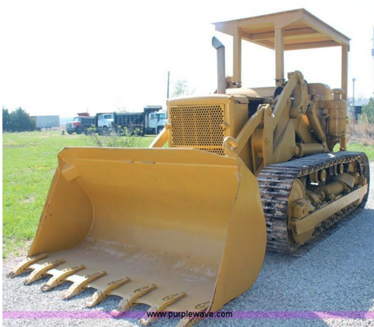
Figure A6: Caterpillar 977H tracked loader. One 977H per crew is anticipated in the plan of operations. (Photo: Purple Wave Auction, https://www.purplewave.com/auction/140515/item/H6548 )
