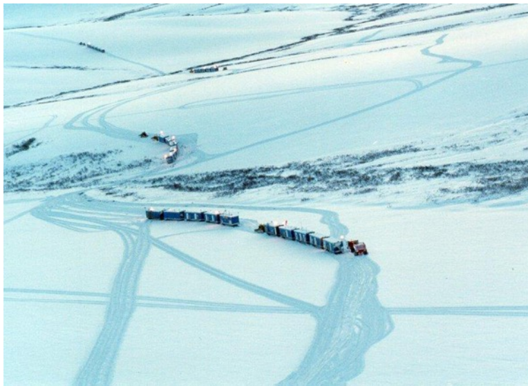
Figure A8: Five strings of Cat trains with sled-mounted camps during 3D seismic exploration in foothills terrain near Kavik, AK, 2001. The three Cat trains in background apparently required two tractors per train to travel in this hilly terrain, while the two in the foreground were waiting for tractors to return for them. (Photo: U.S. Fish & Wildlife Service)
