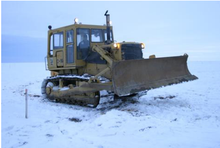
Figure A5: Caterpillar D7 dozer, steel-tracked vehicle used to haul camps and equipment. The plan of operations includes two CAT D7G per crew, but 4 per crew were used at GMT 3D in 2017 and that area was flat, compared to the hilly 1002 where D7s will likely be in high demand. (Photo: Alaska Department of Natural Resources)
