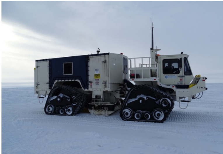
Figure A1: ConocoPhillips rubber-tracked Vibroseis (or "thumper") is a truck-mounted seismic vibrator used to inject low-frequency vibrations into the ground. The vibrator pad is located between the front and rear treads of the vehicle. The plan of operations includes 12 Inova AHV-IV Vibrators per crew. (Photo: Bureau of Land Management)
