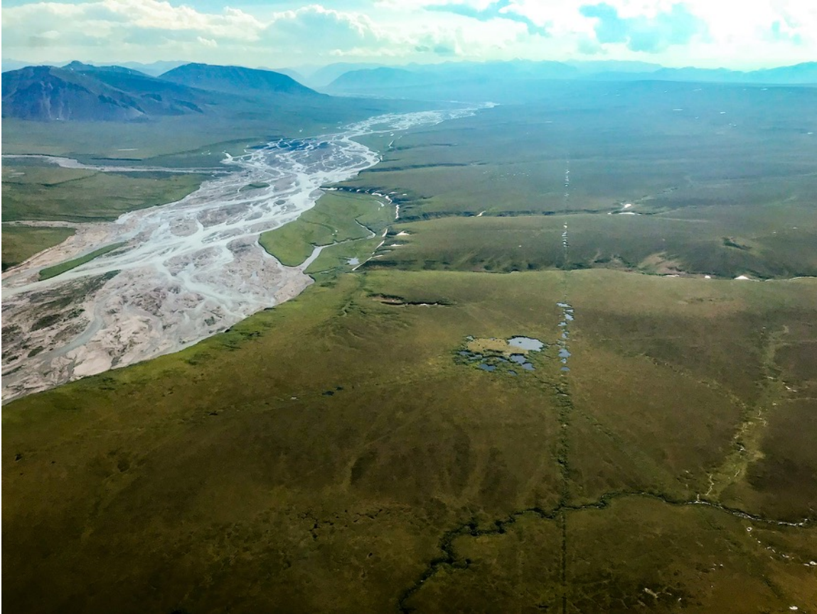
Figure 11. One of many bladed tractor trails just west of the Canning River left from seismic exploration in the 1960s, photographed in 2018. Note the extensive thermokarst and ponding of water along the trail and around the gravel drilling pad near the center of the photo. 48
