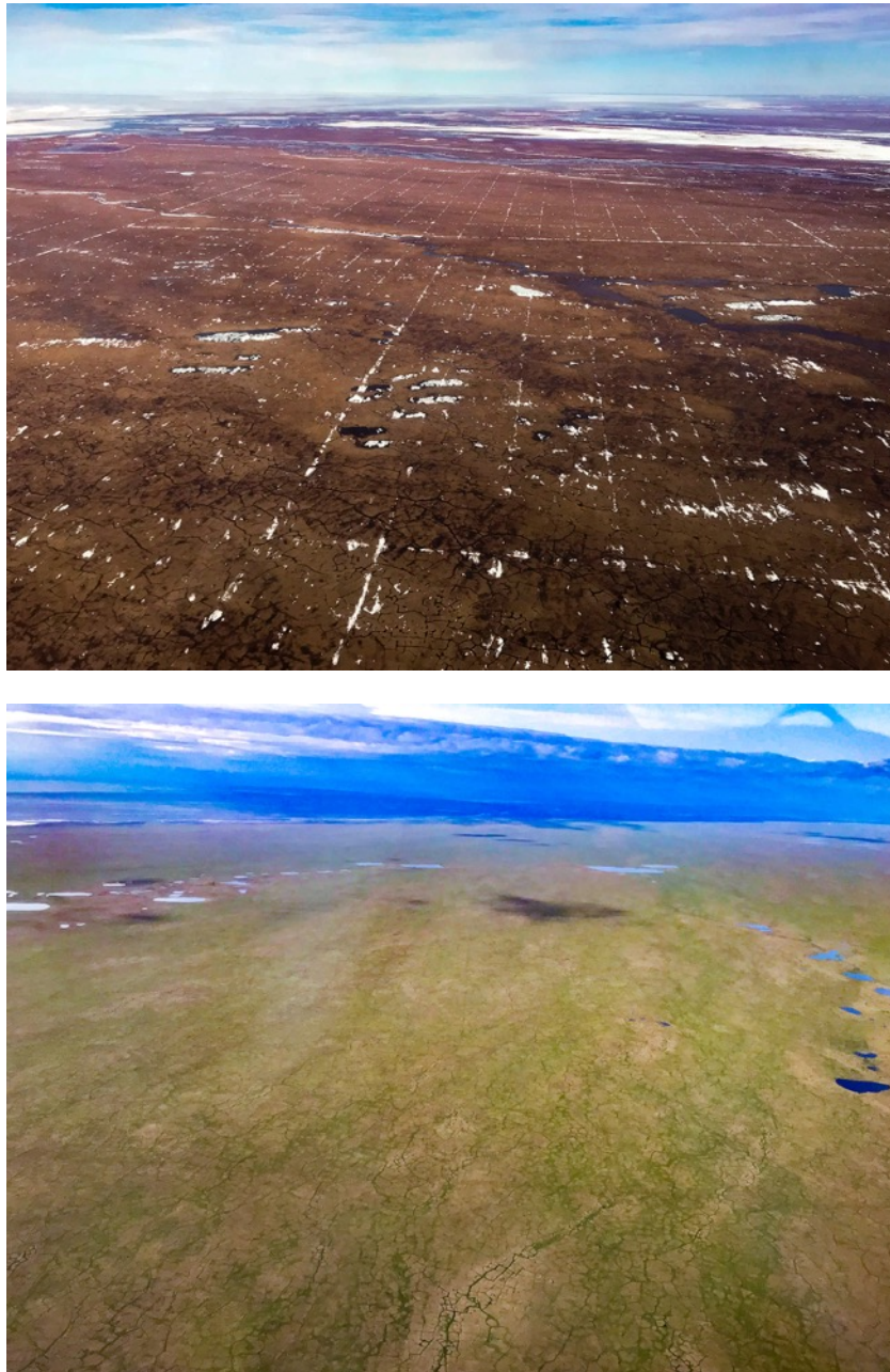
Figure 3. Tracks left by a 3D seismic survey conducted in winter of 2017–2018 on State of Alaska lands along the western boundary of the Arctic National Wildlife Refuge 1002 Area, near the delta of the Canning River. The spacing of the trails is 200 m x 400 m. Top photo shows the grid of trails in early June during snowmelt. 11 The bottom photo shows the trails in midsummer 2018. Although the trails are much fainter in midsummer, they are easily detected because of several factors compared to the adjacent tundra, including differences in the local microtopography (Fig. 7), the amount of standing-dead plant material, and local hydrology (wetter trails). These differences are likely to persist and have long-term ecosystem consequences that will affect the soils, hydrology, permafrost, and plant species. 12
