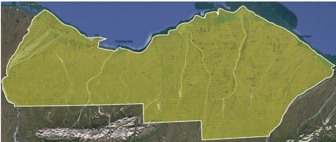
Figure 1. Grid of trails required to do a 3D-seismic survey to cover the entire 1002 Area at 1300-ft (400-m) intervals. 8
