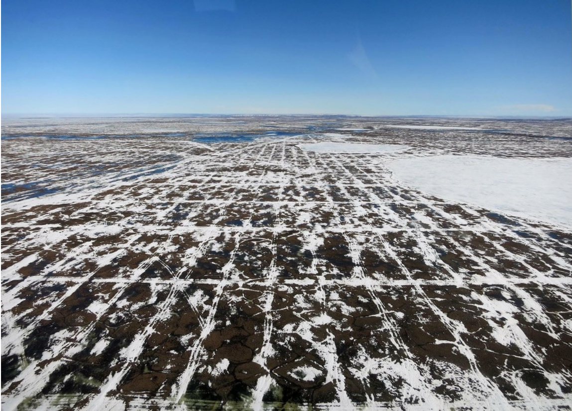
Figure 4. Trails left by the Icewine seismic survey in Spring 2018, approximately 40 km south of the Prudhoe Bay oilfield and 20 km west of the Dalton Highway. The survey consisted of seismic lines spaced 37.5 m to 150 m apart and covered approximately 518 km 2 . 13
