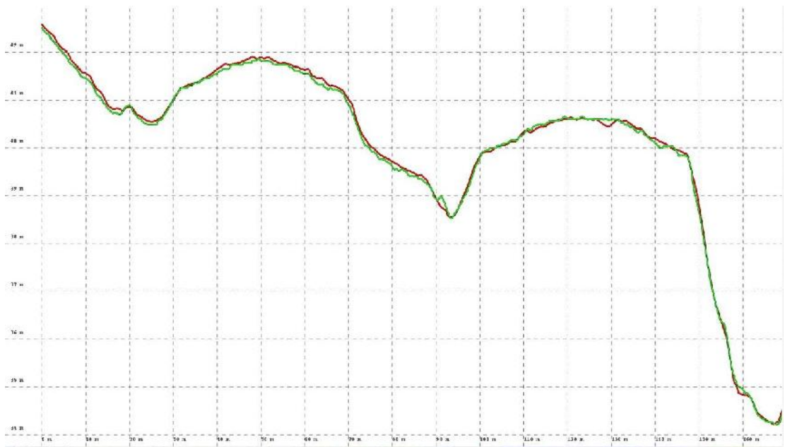
Comparison of Elim village DEM to coastal. The alignment is essentially perfect, with minor differences due to the lower resolution of the coastal data (red). This is the runway and ramp at Elim.
