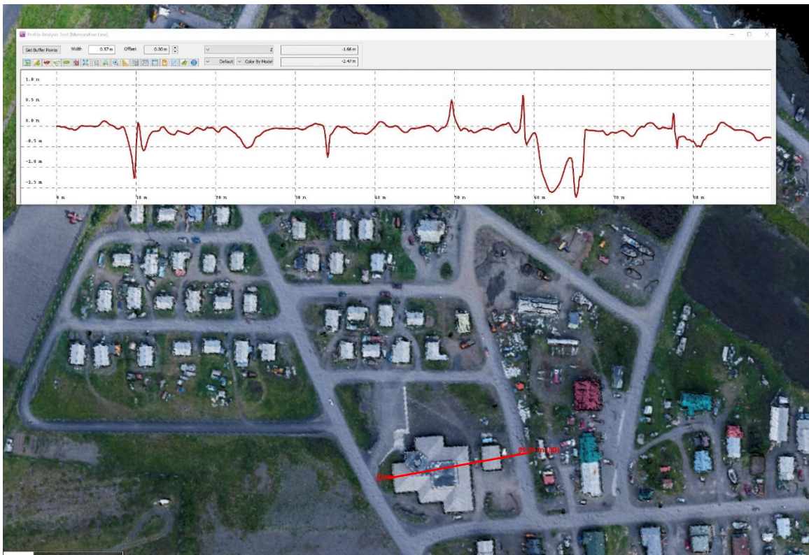
Figure 1 C-D. Another comparison of 2014-2015 Unalakleet data, as in A-B. Here a transect (50 cm vertical ticks) is run across the complex roof of the clinic, which shows no horizontal offsets and a vertical change of essentially zero, as expected. Small spikes are the edges of the buildings, with amplitudes of only \sim 1 m, which is excellent considering the spatial biasing such edges cause. The \sim 1.5 m excursion on the right side is caused by a parked car having moved. Careful examination of the difference image reveals moved boats, cars, snow machines, and small buildings, as well as gravel extraction.
